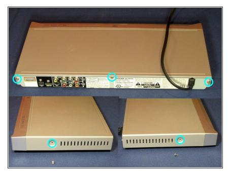
Five identical screws: three in back, one in each of left and right sides.
