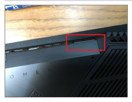
Grasp the back cover where the hinges are for the display.
