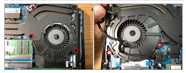
• Remove the screws from the metal cover, lift away from the fan.
