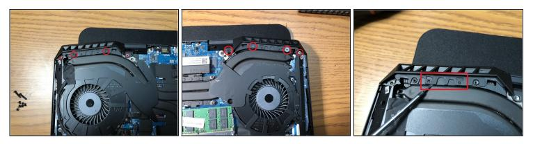
• Remove the four screws from the cover. Insert a flathead screwdriver or a razor blade to lift the cover off the plastic nubs that hold it in place.
