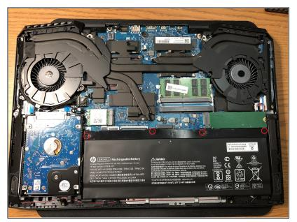
• Remove the 4 screws holding the battery in place. Once removed, pull up on the plastic bar connected to the battery.
