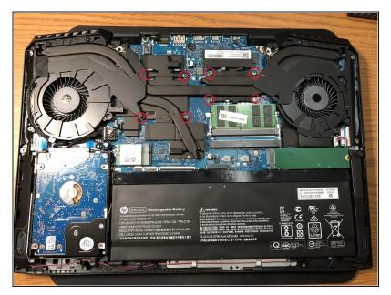
• Remove the 8 screws holding the heatsink to the dies. Note that you need to remove the fan covers first.
