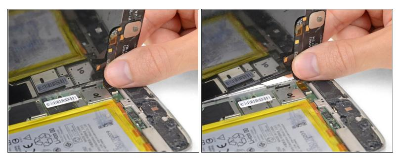
Gently pull the fingerprint sensor cable to slide it out of its socket, disconnecting it from the motherboard.
