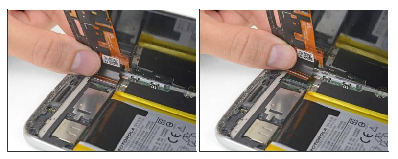
• Gently pull the display cable to slide it out of its socket on the motherboard.
