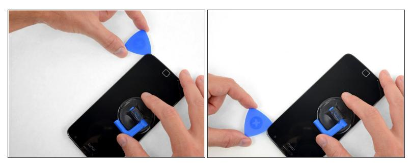
• Slide your tool along the right edge of the phone to separate the glue securing the display.
