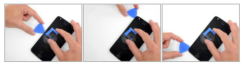
• Slide the tool all along the left edge of the phone to slice through the adhesive securing the display.
