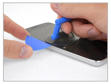
Insert an opening pick (or playing card) into the gap you opened behind the display.
