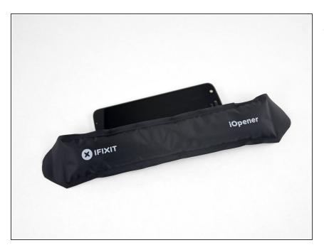
Heat the right edge of the phone to soften the adhesive securing the right edge of the display.
