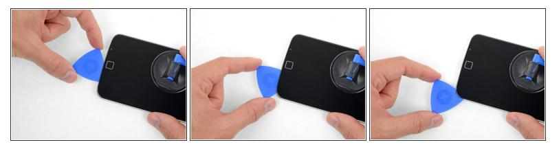
• Continue separating the glue underneath the rest of the lower bezel.
