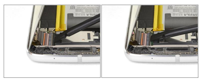
• At the opposite end of the phone, use your spudger to flip open the locking tab on the display cable connector.
