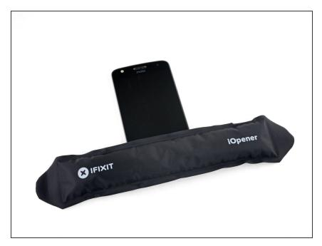
• Heat the front of the phone between the display and the lower edge to soften the adhesive underneath.
