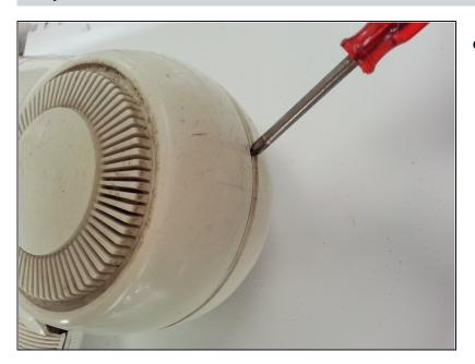
Carefully separate the plastic case with Plastic Opening Tools
