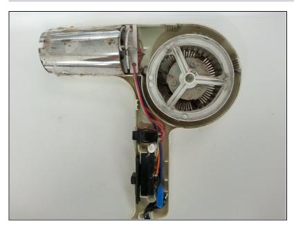
Your hairdryer should now be disassembled and you should easily be able to see the fan, motor, heating element cover, and internal wiring.
