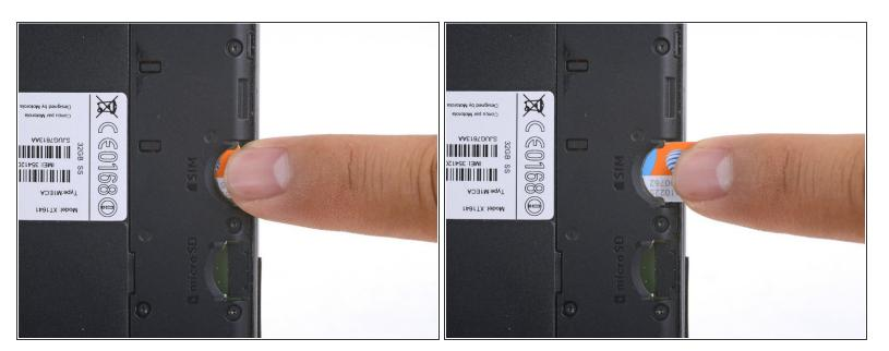
Slide out and remove the SIM card.
