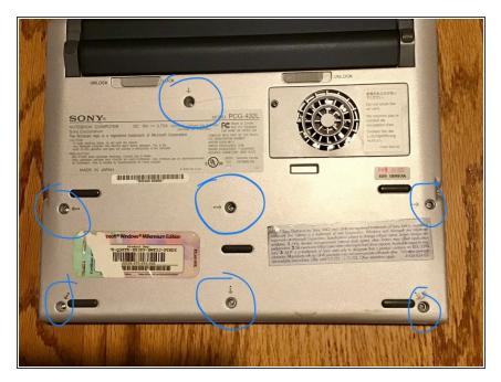
• Remove all circled screws with a Phillips 0 screwdriver. The screw by the top left of the fan does not need to be taken out. Place those screws in a safe place for later.
