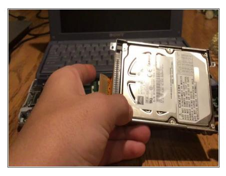
• Grab your old Hard Drive and disconnect the connector on top of the Hard Drive. This may require some force, as seen in the video, but contain the power as to not break the connector!
