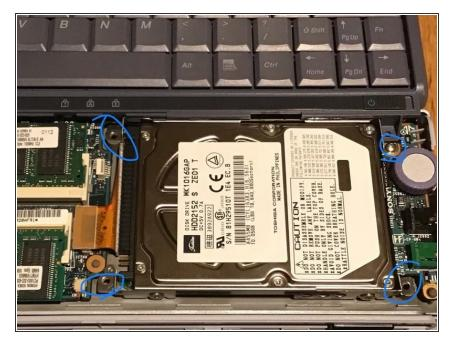
• Unscrew the four screws holding the Hard Drive in place. I am missing some screws so I only have to unscrew one screw, but this may differ for you. Place these screws aside in a safe place for later on.
