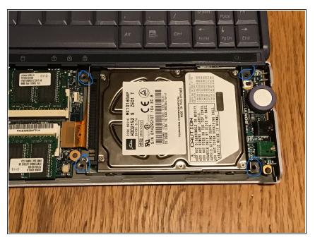
Screw the Hard Drive back into place with a Phillips 0 screwdriver and those screws you put aside earlier for the Hard Drive mount.
