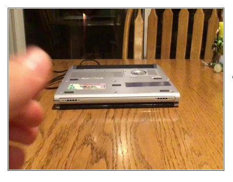
Flip the notebook over, and then unlatch the display. Once that's done, lift up the trackpad and wristrest assembly, but be careful as to lift it up slowly as there is a ribbon cable to disconnect. Once you see the ribbon cable, disconnect it gently with your hands because using pliers can weaken the integrity of the cable. Put the assembly aside.
