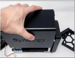
Once the rear panel is removed, the housing can be removed. To do so drag the cover about 1 cm to the back of the NAS then lift the hood upwards.
