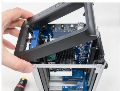
and remove the front panel ...
