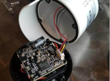
Remove the 4 screws holding down the camera lens. They are standard Philipps #1
