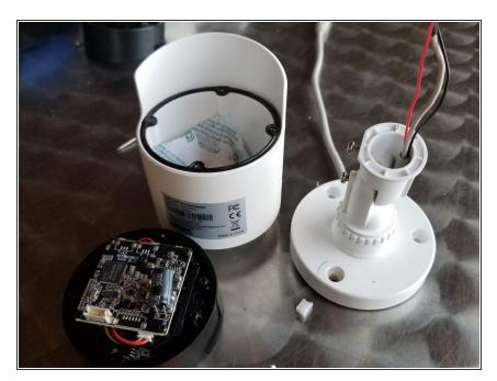
Very simple design for a very simple device. The whole assembly is held by 6 screws. Making it very easy to re-assemble.
