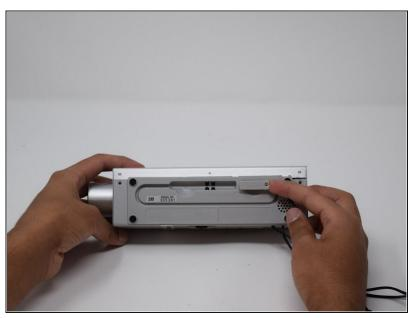
• Remove the battery cover tab.
