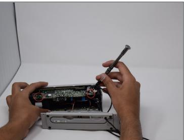
• Remove screws from motherboard as shown in the photo.
