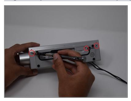
Remove the screw from the backside cover of the recorder with a Phillips Screwdriver.
