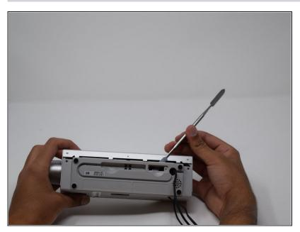
Remove the backside cover of the device. You can pry open with a screwdriver if necessary.
