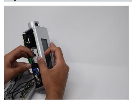
• Remove the paper tab from its slot and re-insert it.
