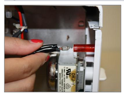
• Reinsert the indicator light back into the red tube.
