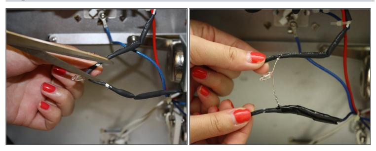
• Use scissors to cut open cord sheathing and peel back.
