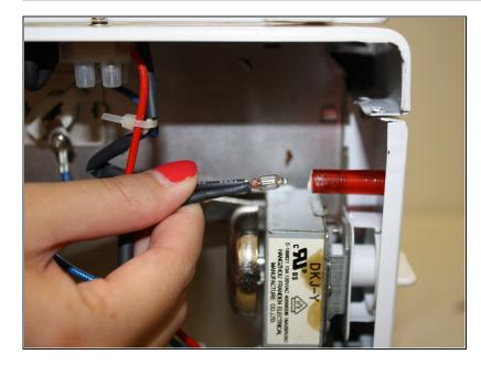
• Pull the black wires to remove the indicator light from the red tube.
