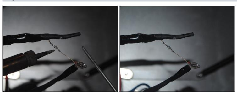
• Solder the replacement light bulb back onto its original position.
