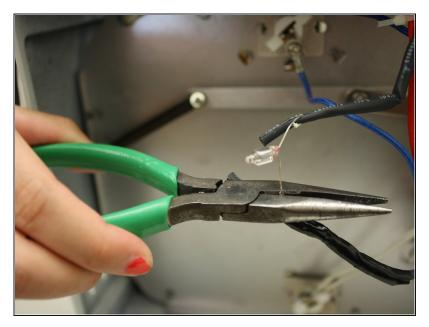
• Use the wire-cutters to remove the light bulb.
