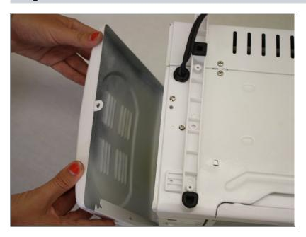
• Remove the panel on the left hand side. The indicator light is located in the red tube that has wires covered by black tubing coming out.
