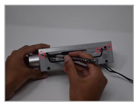
Using a Phillips #0 screwdriver unscrew the three screws that connect the back panel to the device.
