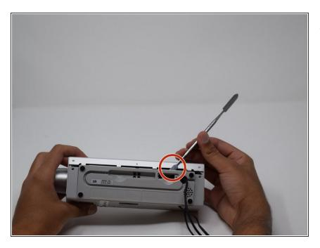
Using a thin flat tool, pry off the panel on the back of the device.
