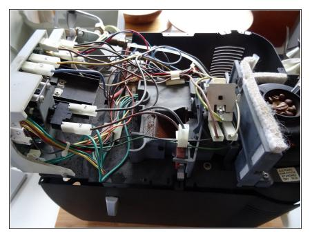
It's safer to number the cable connectors on the electronics. You probably just need to disconnect the slightly hidden # 14 connector on the two green cables at the very bottom and # 7 on the blue cable on the top.
