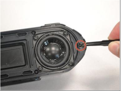
• Use the tweezers to remove the six rubber stoppers. There are four in the middle and two on the sides.
