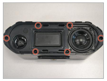
Use the PH1 Phillips screwdriver to remove the six 12mm screws that lie underneath each rubber stopper.
