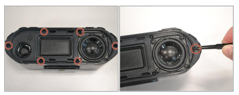
• Use the tweezers to remove the six rubber stoppers. There are four in the middle and two on the sides.
