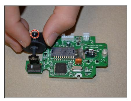
Push the scroll wheel to the right side of the motherboard as shown, then pull it away from the board to remove.
