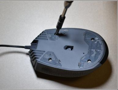
Use the JIS 0 screwdriver to remove the four 5 mm screws on the bottom of the mouse.
