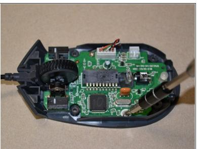
Use the JIS 0 screwdriver to remove the two 5mm screws on the motherboard.
