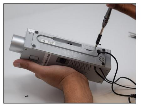
To start, use a small phillips screwdriver, to remove the screw located on the battery component on the back of the device.
