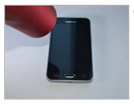
Apply heat from heat gun or blow dryer on periphery of the screen for one to two minutes.
