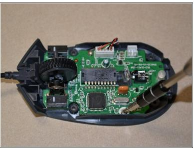
Use the JIS 0 screwdriver to remove the two 5mm screws on the motherboard.
