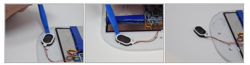
• After the connections are desoldered, remove the speaker by prying it up using a plastic opening tool.
