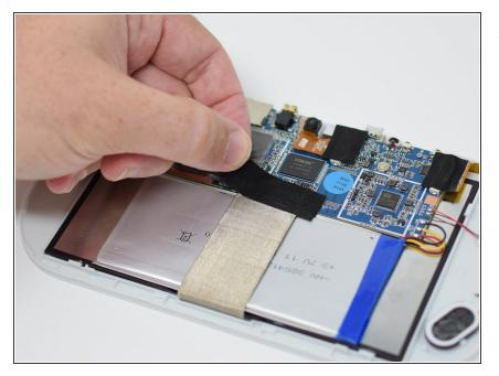
• Remove the black tape to reveal the wire ribbon connector.
