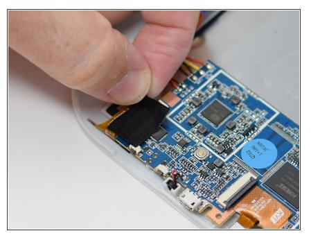
• Remove the black tape to reveal the screen connector.
