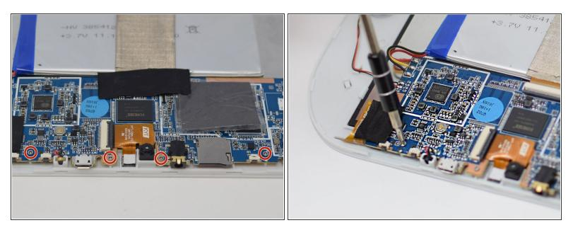
Using a PH 00 screwdriver, remove the four 4.5 mm screws that are holding the motherboard in place.
