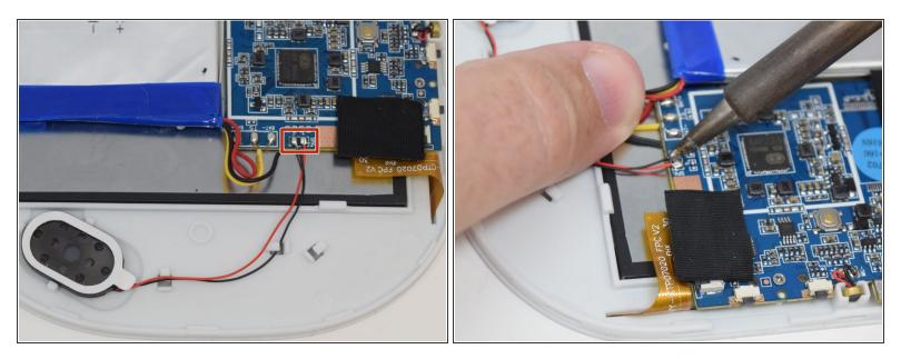
Remove the wires from the motherboard using a soldering iron tool. Here is a link on <u>How To</u> <u>Solder and Desolder Connections</u>.
