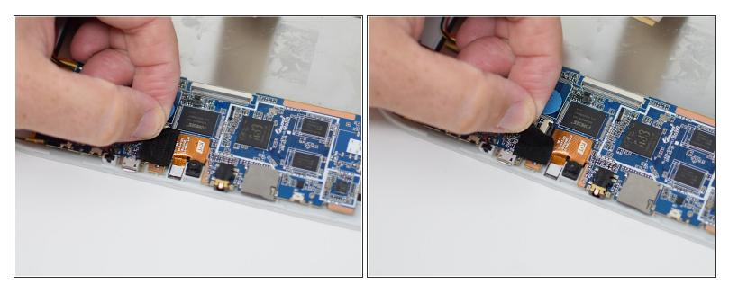
• Remove the black tape to reveal the wire ribbon connector.
