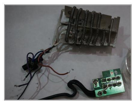
The heating element assembly will now be separated from the circuit board and can be replaced with a new one.
