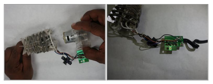
Once the fan/motor assembly is disconnected from the heating element assembly you will see that the heating element assembly is connected to a circuit board by four wires. The color of these wires are grey, black, purple and brown.
