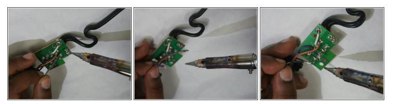
• Desolder these four wires one by one from the circuit board.
