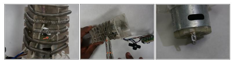
• The fan/motor assembly is connected to the heating element assembly at two points need to be desoldered. After pulling the attached wires through the holes the fan/motor assembly will be free from the heating element assembly. Congratulations you have now completely removed the fan/motor assembly from this hair dryer!
