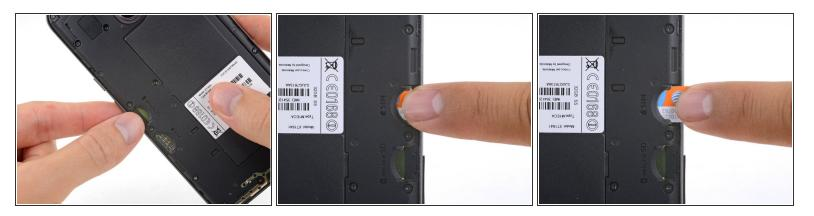
Push to eject and remove the MicroSD and SIM cards (if installed).
