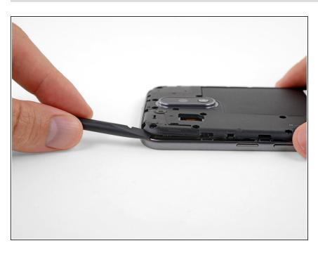
Insert a spudger under the midframe at the top left corner, and gently twist to separate it from the body of the phone.
