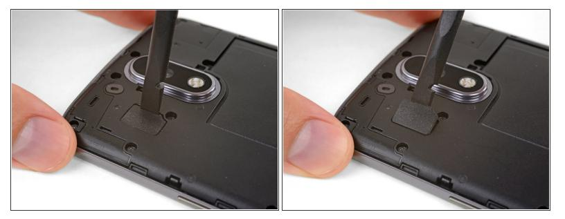
• Use a spudger to pry up the rubber cover for the camera flash connector.
