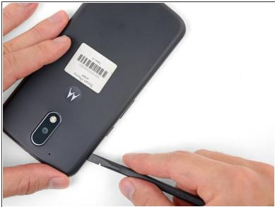
Slide your tool all along the side of the phone to separate more of the clips securing the back cover.
