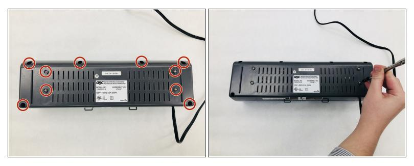
• Using the Phillips #2 screwdriver, remove ten 12 mm long screws on the bottom of the device.
