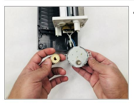
• Pull the gear off of the motor.
