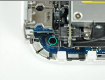
• Remove the Phillips screw near the audio ports securing the internal frame to the bottom case.
