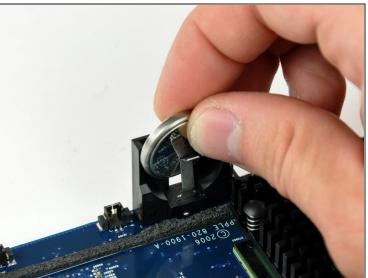
• Push the PRAM battery toward the center of the logic board and pull it up out of its holder. You'll have to push the battery in further than you'd expect in order to get it to pop free.
