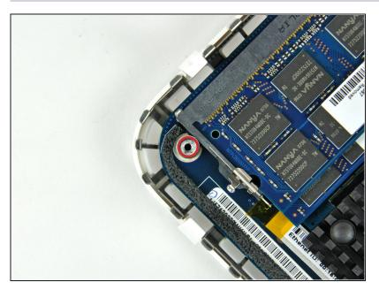
Remove the single T10 torx lug securing the logic board to the bottom housing.
