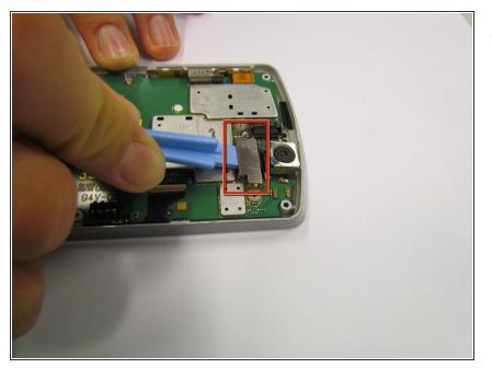
• Use the plastic opening tool to lift the camera from the phone.
