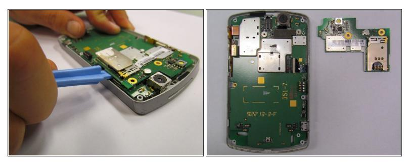
Remove the glued, mounted surface by lifting it from underneath the SIM card slot by using the plastic opening tool.
