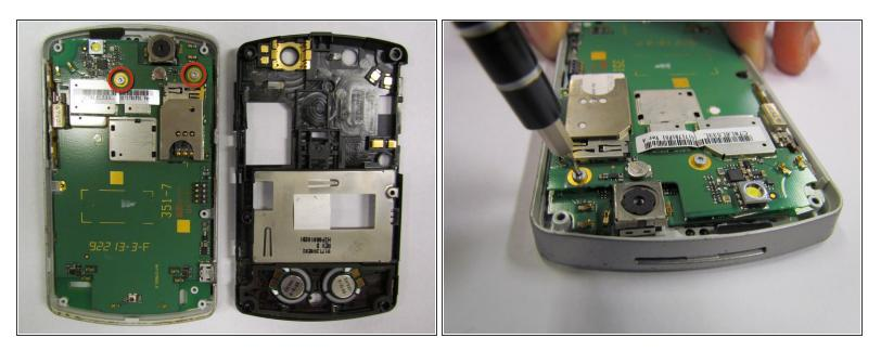
• Remove both screws on the mounted surface with a T5 screwdriver.
