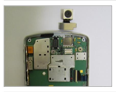
• The new camera can now be attached to the motherboard.
