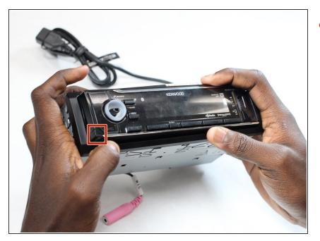
• Press the ejection button on the lower left corner of the face plate.
