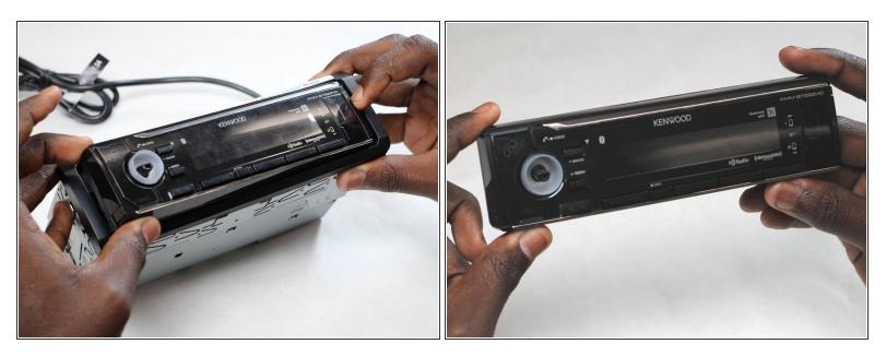
• Remove the face plate by pulling upwards and in the direction of the ejection button.
