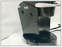
Remove the water reservoir from the Keurig machine by gently lifting up on the reservoir and pulling it away.
