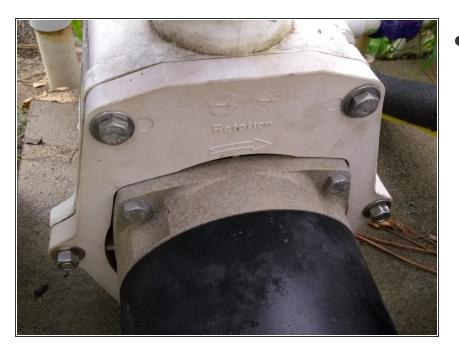
There are four 9/16" bolts two upper (visible) and two lower (not visible) in my photo. Also there are two 9/16" nuts with bolts visible in the photo as the middle part that holds the pump housing halves together.
