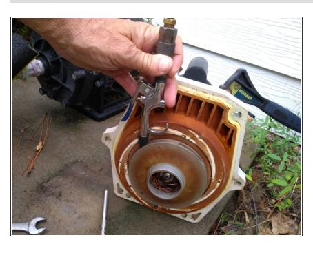
Apply compressed air into each impeller outlet vane as shown in the photo. You will want eye protection here!!! Now you are ready to reassemble in reverse order of the above steps. Don't forget to add water into pump chamber before powering up pump!
