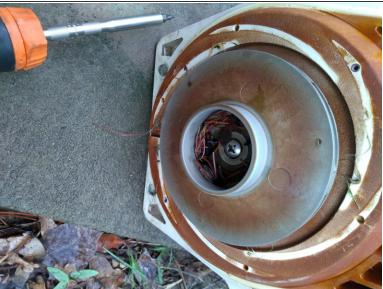
• This is held in place by two tiny allen head machine screws (3/32"). These are visible in the first image here (impellor cover removed). Pull off the cover and set aside for now. 2nd Pic shows the rather obvious problem of the debris in intake chamber of impeller after the cover is removed.
