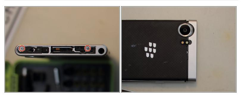
• Remove the two Philipps #0 screws that hold in place the top of the phone frame and slide it off.
