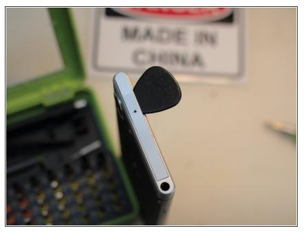
Carefully remove the top plastic cover. It is hold in place by adhesive.
