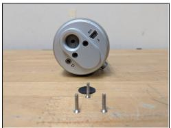
First remove the Rubber inside the screwable mount area. This can easily be done with a small screw driver tip or Tweezers. From here you can remove the 3 screws using a #1 Phillips head.
