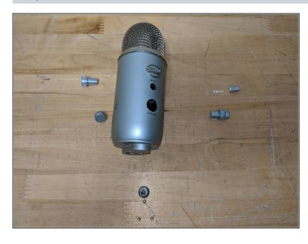
The 4 exterior buttons can be removed with any force such as fingers or any form of pliers. I used my fingers to remove and pull the buttons from their button placement. You will notice there is a lot of give from the mesh and the body.
