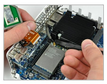
Use the flat end of a spudger to pry the AirPort antenna cable connector up off the AirPort card.
