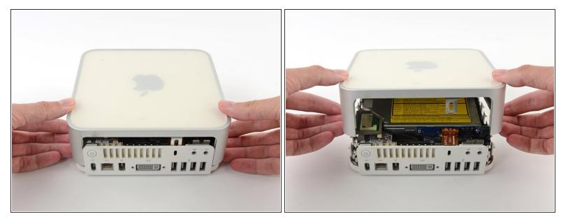
Flip the Mac mini back over and lift the top housing off of the lower housing.
