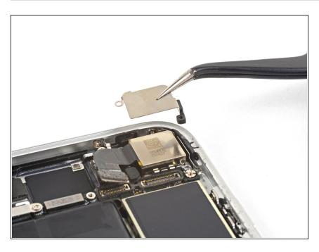
Remove the rear-facing camera bracket.
