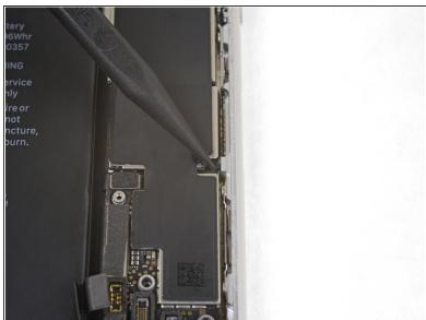
Use the point of a spudger to move the SIM card eject plunger out of the logic board's way.
