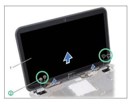
Replace the screws that secure the display assembly to the computer base.
