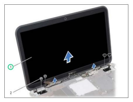
Place the NEW display assembly on the computer base and align the screw holes on the display assembly with the screw holes on the computer base.
