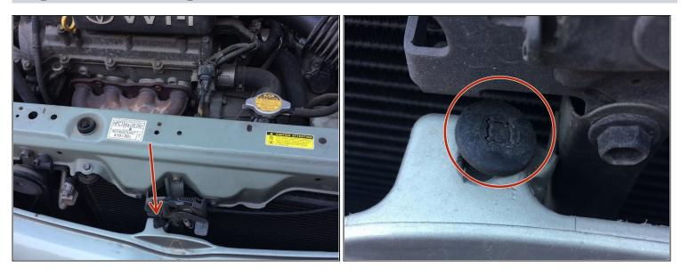
• Release the plastic clip which attaches the top of the bumper to the middle of the radiator grill.
