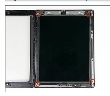
Remove the four 2 mm Phillips #00 screws securing the LCD to the aluminum frame.
