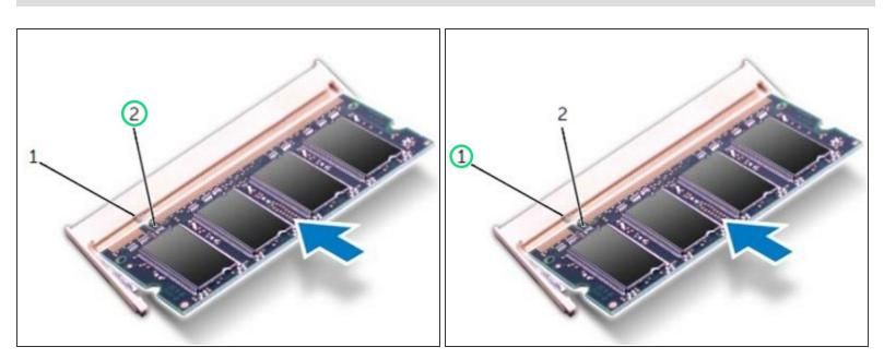
• Align the notch on the **NEW** memory module with the tab on the memory-module connector.
