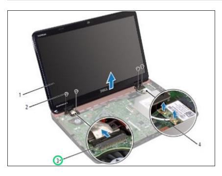
Connect the display cable and touch-screen cable to the connectors on the system board.
