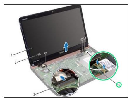
Note the routing of the Mini-Card antenna cables and remove the cables from the routing guides.
