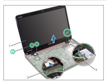
Remove the four screws that secure the display assembly to the computer base.
