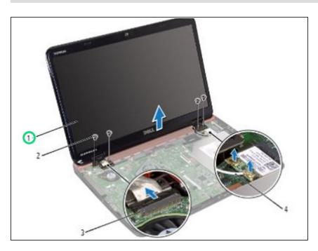
Place the **NEW** display assembly in position and replace the four screws that secure the display assembly to the computer base.
