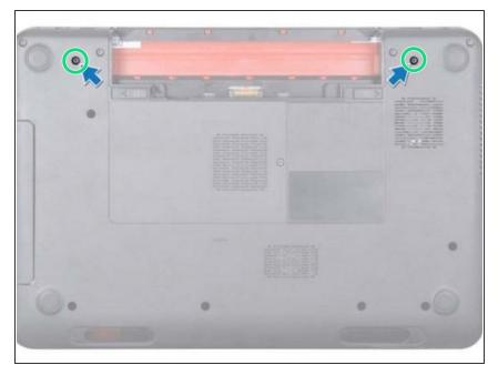
Replace the two screws that secure the display assembly to the computer base.
