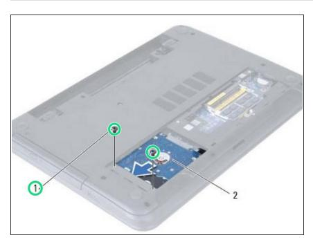
Remove the screws that secure the hard-drive assembly to the computer base.
