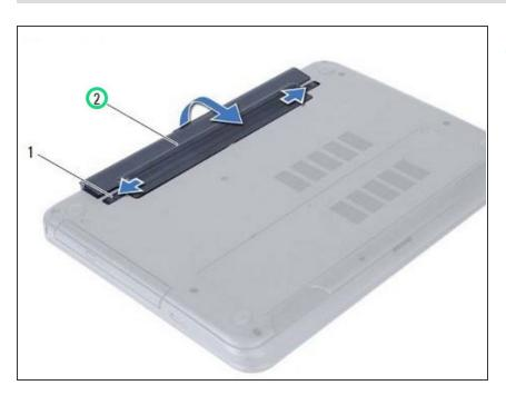
Lift and remove the battery off the computer base to disconnect it from the computer.
