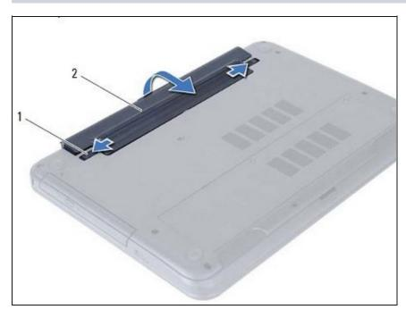
Align the tabs on the battery with the slots on the battery bay and snap the battery into place.
