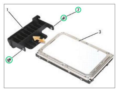
Remove the two M3 x 3-mm screws from each side of the hard drive bezel, then pull to separate the bezel from the hard drive.
