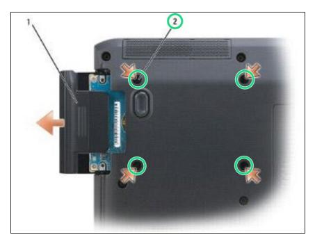
Replace the four M3 x 3-mm screws to secure the hard drive.
