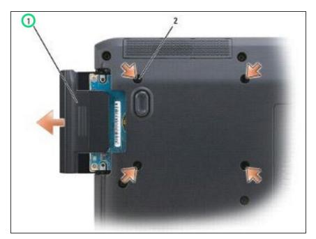
Slide the hard drive into the hard drive bay until the drive is fully seated.
