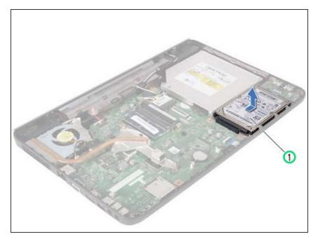
Slide the hard drive to the right to disconnect it from the connector on the system board.
