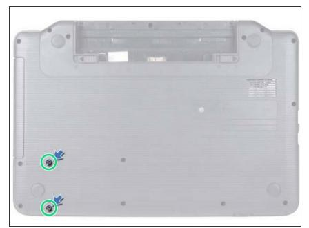
Replace the two screws to the computer base.
