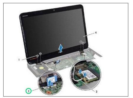
Disconnect the display cable from the connector on the system board and remove it from the routing guide.
