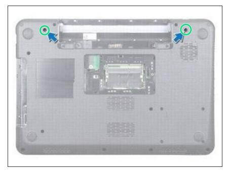
• Turn the computer over and replace the two screws at the bottom of the computer.
