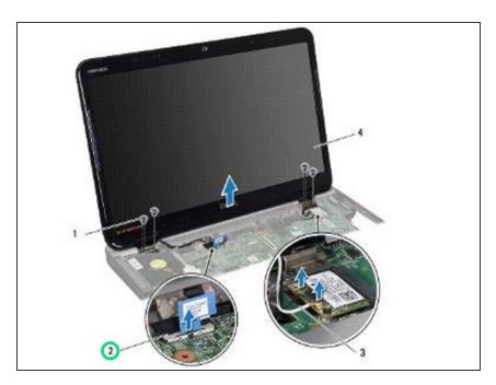
Route the display cable into the routing guide and connect the cable to the connector on the system board.
