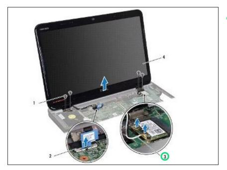
Connect the Mini-Card antenna cables to the connectors on the Mini- Card.
