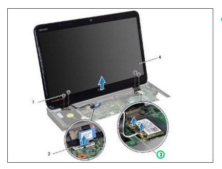
Disconnect the Mini-Card antenna cables from the Mini-Card.
