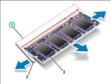
Use your fingertips to carefully spread apart the securing clips on each end of the memory-module connector until the module pops up.
