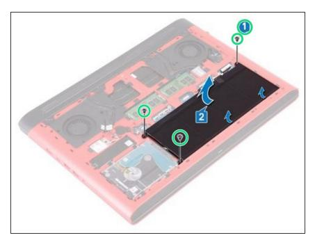
Replace the three screws (M2.5x6) that secure the battery to the computer base.
