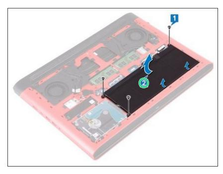
Slide the **NEW** battery in the slot on the computer base and align the screw holes on the battery with the screw holes on the computer base.
