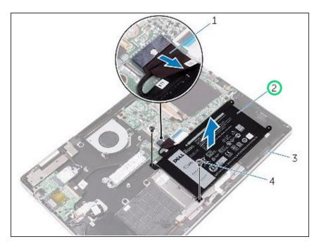
Lift the battery along with the battery cable off the palm-rest assembly.
