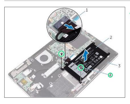
Remove the screws that secure the battery to the palm-rest assembly.
