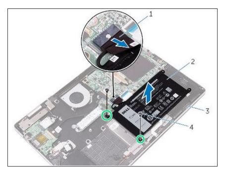
Align the screw holes on the NEW battery with the screw holes on the palm-rest assembly.
