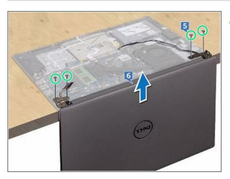
Remove the four screws (M2.5x5) that secure the display hinges to the palm rest and keyboard assembly.
