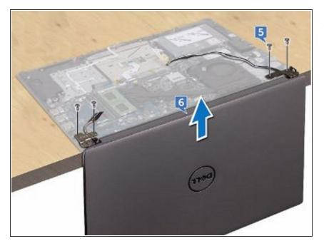
Place the palm rest and keyboard assembly on the edge of a table with the keyboard facing down.
