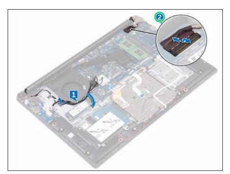
• Open the latch and disconnect the display cable from the system board.
