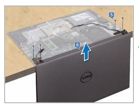
Place the computer on the edge of a table so that the palm rest and keyboard assembly is on the table
