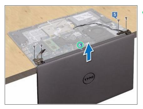
Open the display at an angle of 90 degrees.
