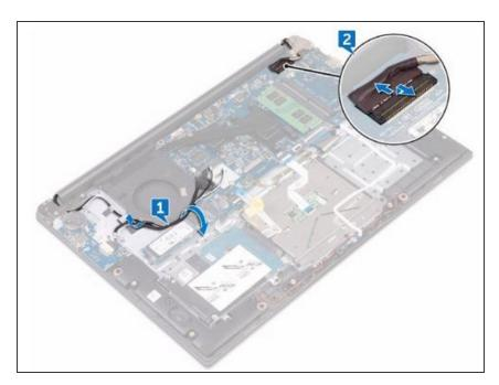
• Route the antenna cables through the routing guides on the fan.
