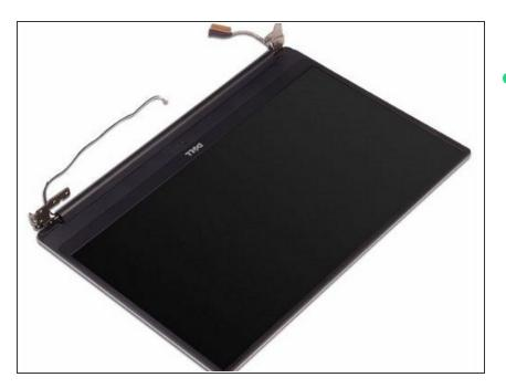
Lift the display assembly off the palm rest and keyboard assembly.
