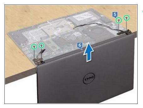
Replace the four screws (M2.5x5) that secure the display assembly to the palm rest and keyboard assembly.
