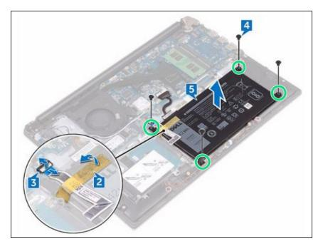
Align the screw holes on the NEW battery with the screw holes on the palm rest and keyboard assembly.
