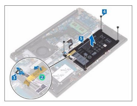
Adhere the tape that secures the hard-drive cable to the battery.
