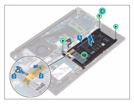
Replace the four screws (M2x3) that secure the battery to the palm rest and keyboard assembly.
