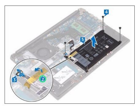
Peel the tape that secures the harddrive cable to the battery.
