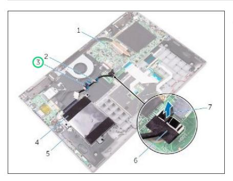
Peel off the tape that secures the hard-drive cable to the palm rest and keyboard assembly.
