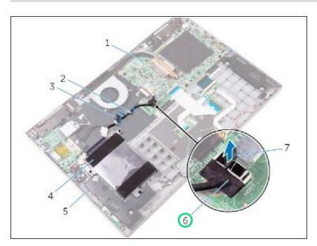
Note the hard-drive cable routing and remove the cable from the routing guides.
