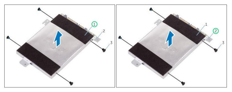
Lift the hard drive off the hard-drive bracket.
