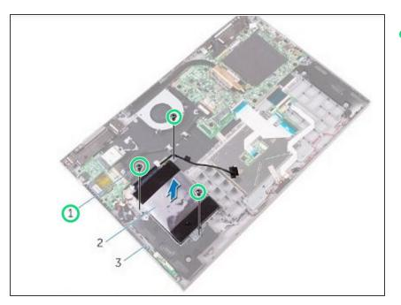
Remove the three screws (M2x3) that secure the hard-drive assembly to the palm rest and keyboard assembly.
