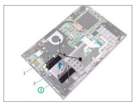
Route the hard-drive cable through the routing guides on the palm rest and keyboard assembly.
