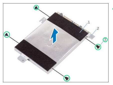
Replace the four screws (M3x3) that secure the hard-drive bracket to the hard drive.
