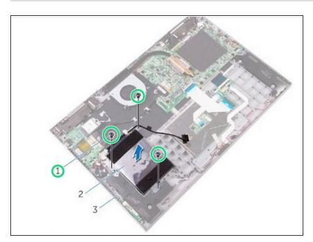
Replace the screws three (M2x3) that secure the hard-drive assembly to the palm rest and keyboard assembly.
