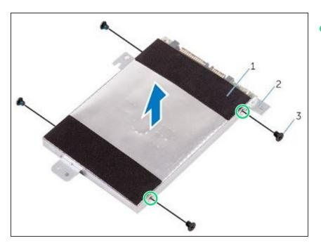
Align the screw holes on the NEW hard-drive bracket with the screw holes on the hard drive.
