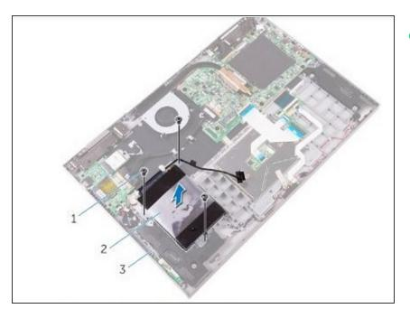
Adhere the tape that secures the hard-drive cable to the palm rest and keyboard assembly.
