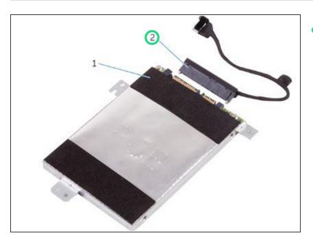
Disconnect the interposer from the hard-drive assembly.
