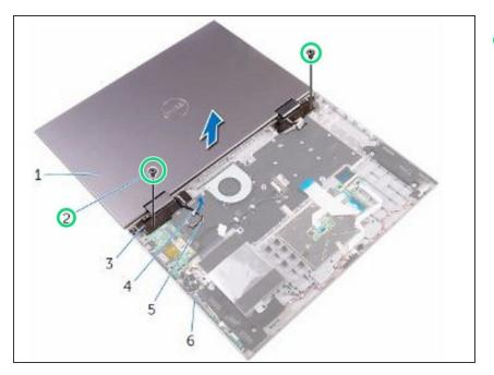
Remove the screws that secure the display assembly to the palm rest and keyboard assembly.
