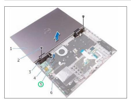
Remove the antenna cables from the routing guide on the palm rest and keyboard assembly.
