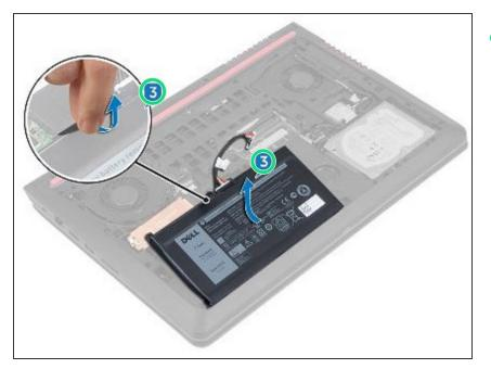
Using the pull tab, lift the battery, along with its cable, off the computer base.
