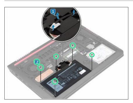
Remove the five screws (M2x5 T8) that secure the battery to the computer base.
